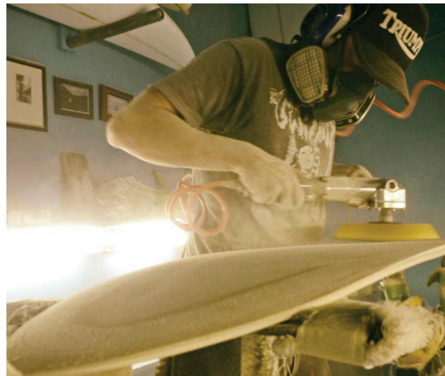
Chris and Jeremy hand shaped the outline and rocker profile of the Storm Chaser and Mountain Surfer using Chris' surf shaping tools. Photo Left/ Top - Seth Lightcap, Bottom Jeremy Jones
