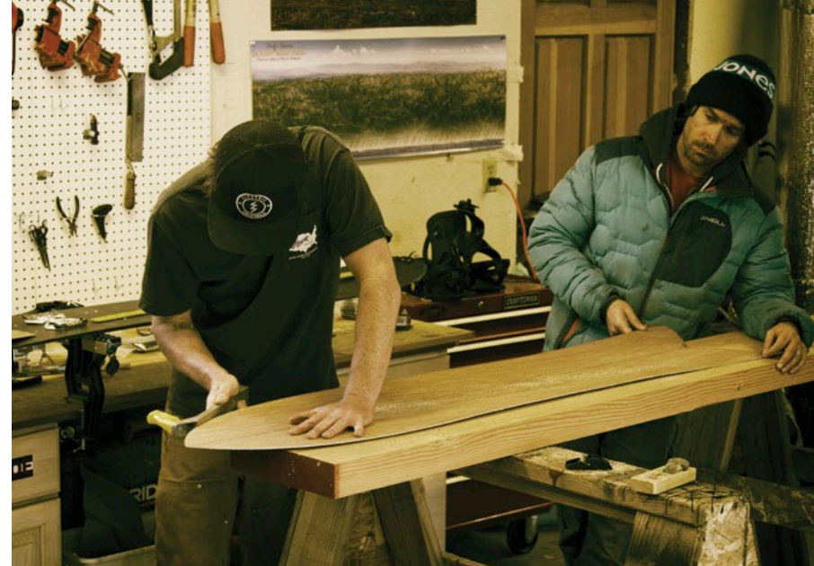
Chris and Jeremy hand shaped the outline and rocker profile of the Storm Chaser and Mountain Surfer using Chris' surf shaping tools. Photo Left/ Top - Seth Lightcap, Bottom Jeremy Jones
