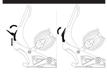
This type of binding's forward lean block allows four settings: 0 mm, +4 mm, +8 mm and +12 mm. The factory setting is 0 mm / +12mm. Switch between these two settings by spinning the block. To change to +4 mm / +8 mm settings, unscrew the block from highback, flip the small plastic piece and
