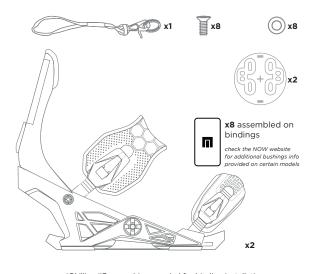
\*Phillips #3 screwdriver needed for binding installation.
