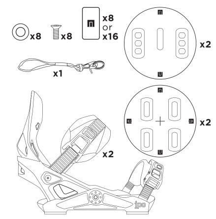
\*Phillips #3 screwdriver needed for binding installation.
