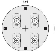
**PLEASE NOTE:** Slotted holes are offset from disc center marked with a **+**
